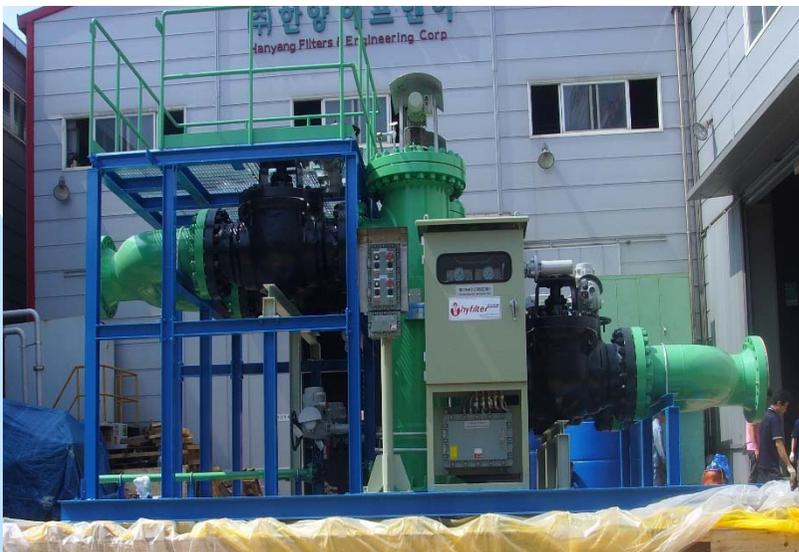
It is a system composed of two automatic strainers of the basket type. Individual operation, cross operation, and simultaneous operation are possible to fully guarantee the stability of the process.
