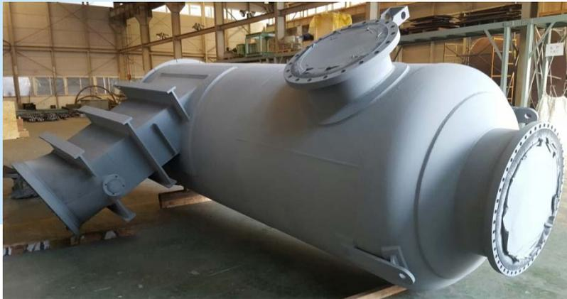
It is a device that removes liquid mist or impurities in gas or gas.
