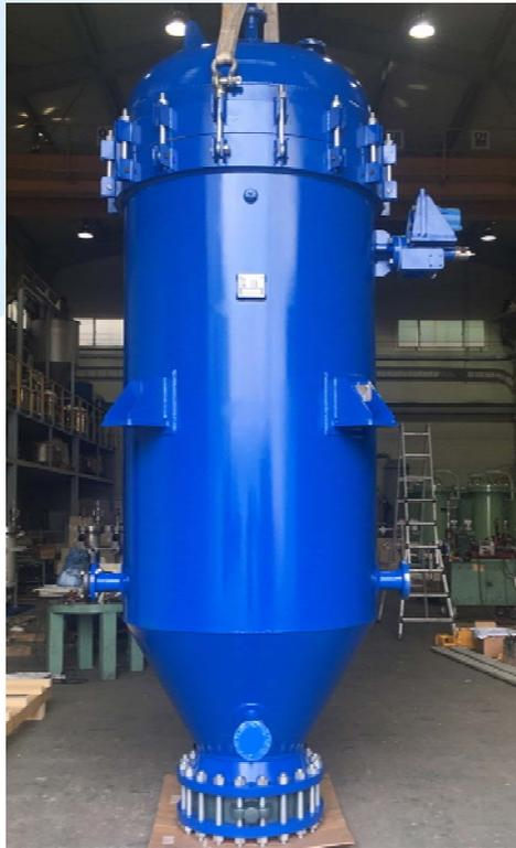
It is a device that filters the cake by individually mounting leaf-shaped filter elements in a vertical housing on the central manifold.
