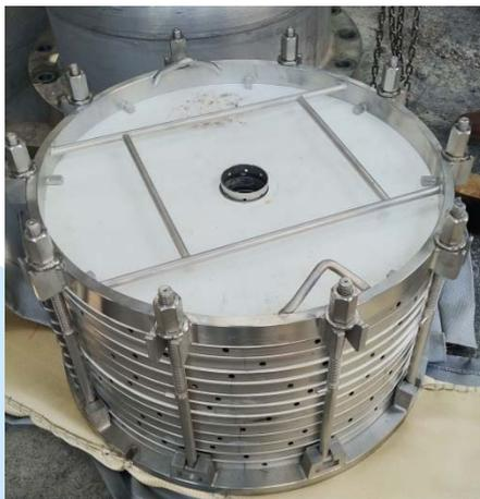
It is a device that filters by stacking a male circular type filter plate.
