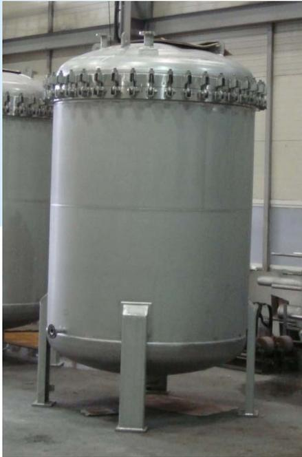
It is a filtration device that individually mounts a bag-type filter media on the upper manifold and pre-coats it.
